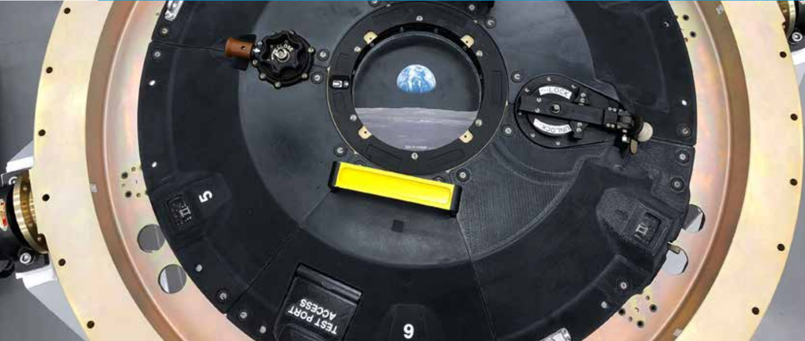
The Orion docking hatch cover 3D printed with Antero™ (ESD).
