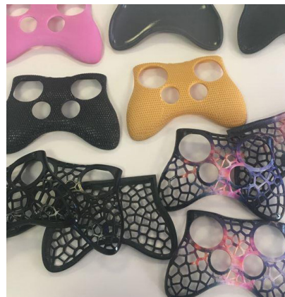
Figure 1: With the J Series, it only took a single five-hour print to produce a multimaterial controller prototype, with rigid VeroWhite™ for the body and rubberlike Agilus30™ for the buttons.
