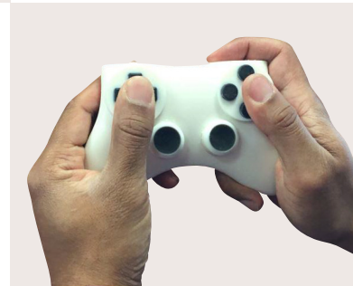
Figure 1: With the J Series, it only took a single five-hour print to produce a multimaterial controller prototype, with rigid VeroWhite™ for the body and rubberlike Agilus30™ for the buttons.
